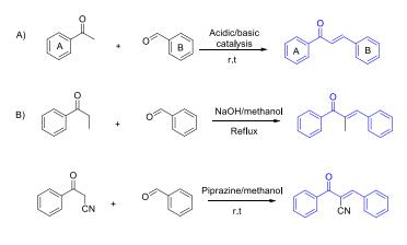
Scheme 1: A) Traditional Claisen–Schmidt condensation. B) Examples of modified temperature conditions.
