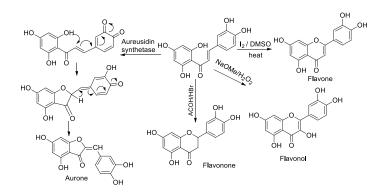
Scheme 11: Chalcone isomerization into flavone, flavonol, flavonone and aurone.
