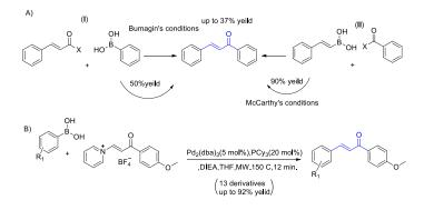
Scheme 2: chalcone synthesis via A) Suzuki coupling different approaches B) Suzuki-Miyaura reaction applications.
