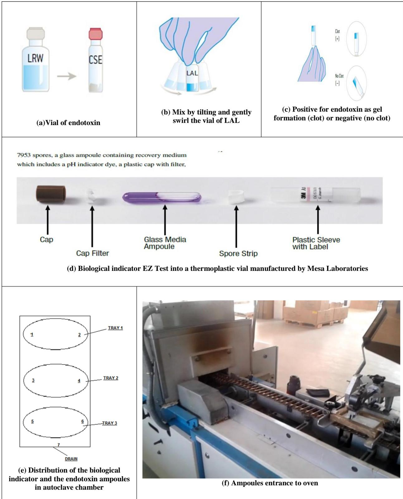
Plate I. Sterilization and depyrogenation tests
